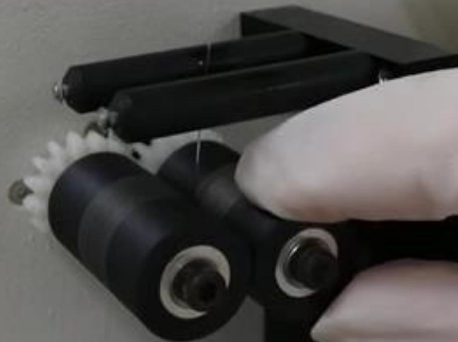
④Route the ribbon through the guide and roller to prevent it from twisting.
