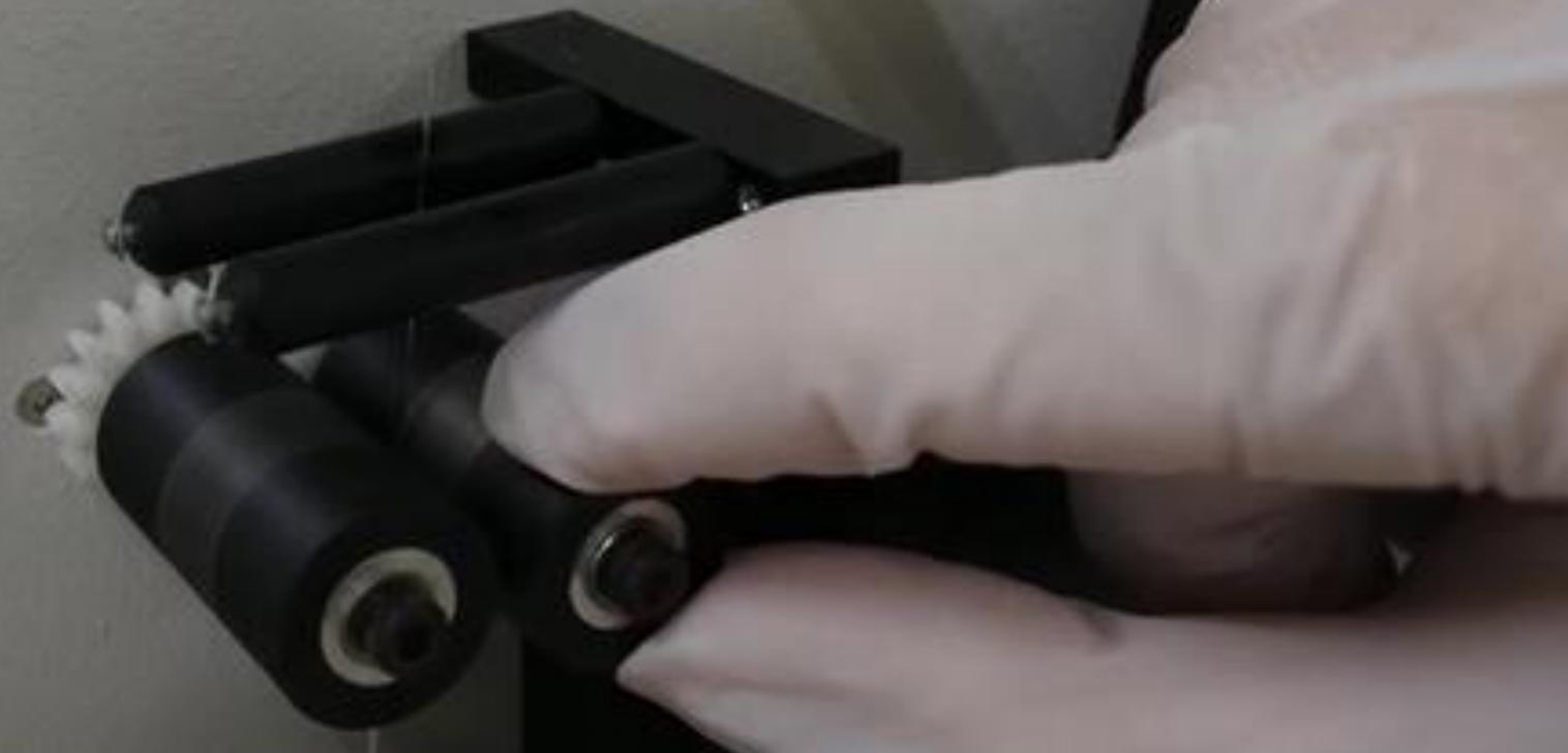
④Route the ribbon through the guide and roller to prevent it from twisting.
