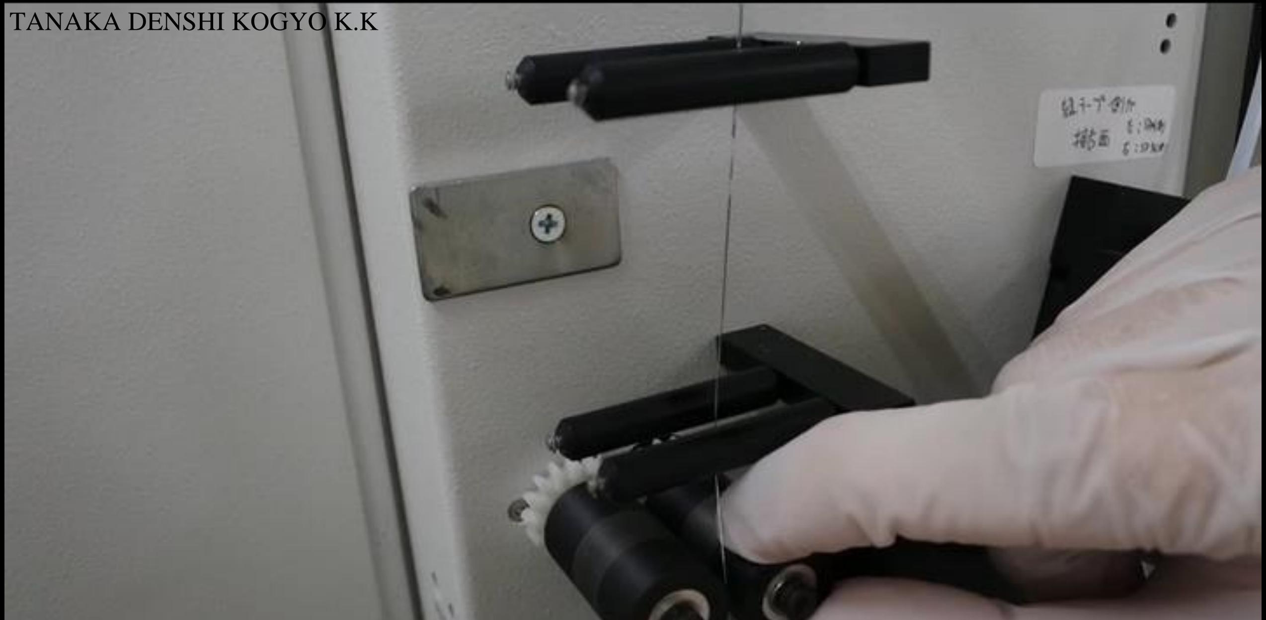
④Route the ribbon through the guide and roller to prevent it from twisting.
