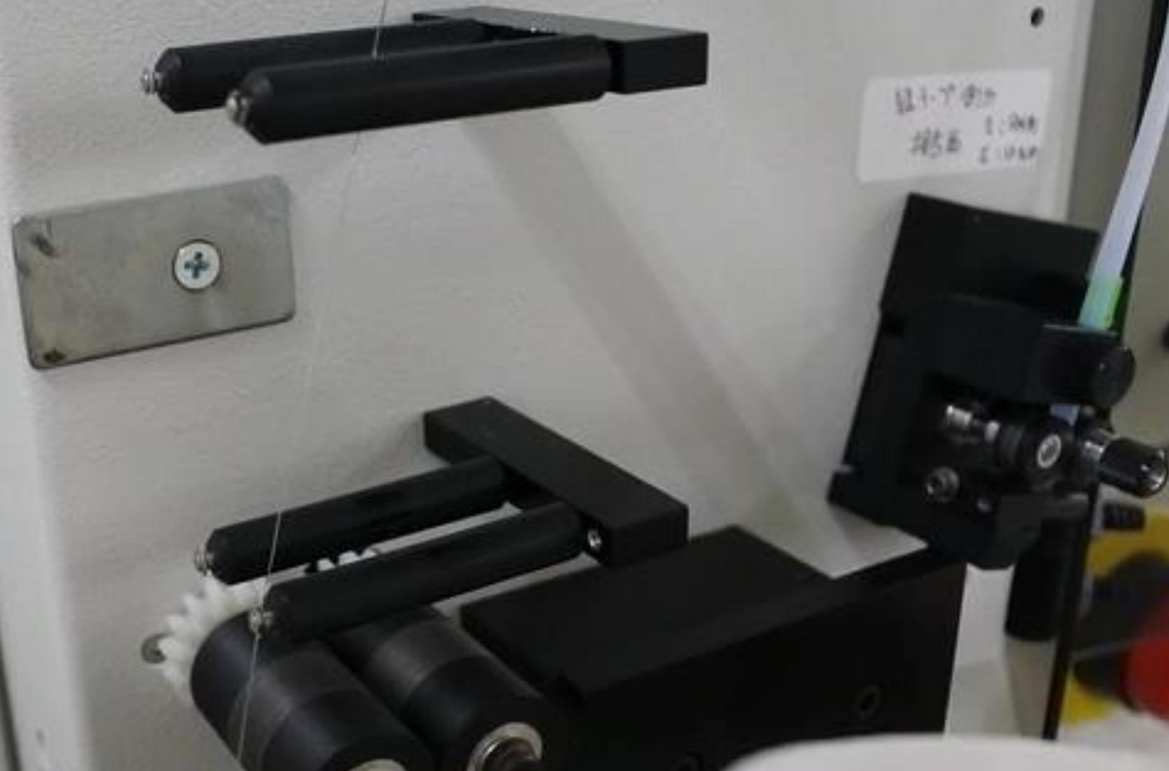
④Route the ribbon through the guide and roller to prevent it from twisting.
