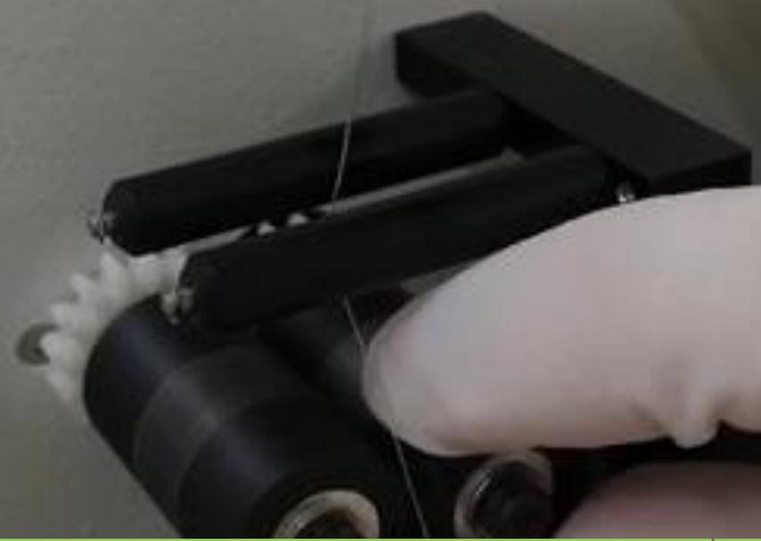
④Route the ribbon through the guide and roller to prevent it from twisting.
