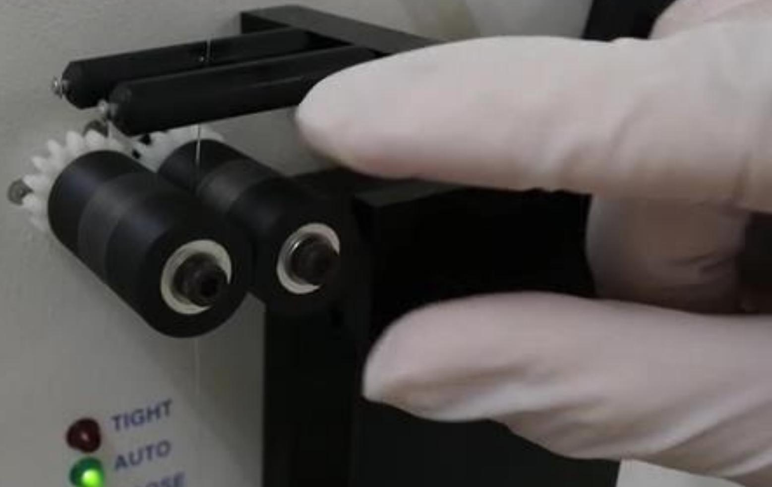
④Route the ribbon through the guide and roller to prevent it from twisting.
