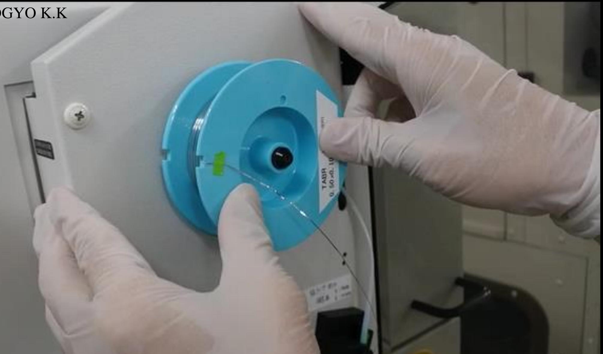
① Set the spool removed from the case to the bonding machine.
